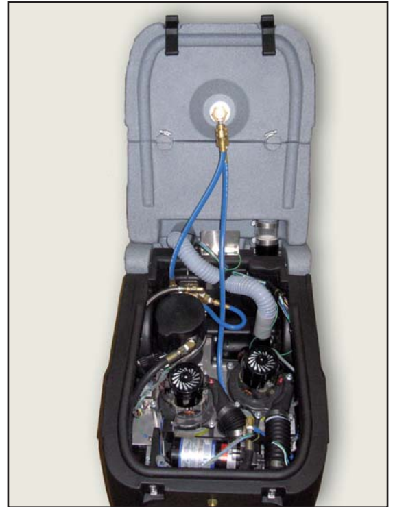
Two 2-stage vacuum motors, 7 bar pump, and a 2-stage in-line heater with 2000 Watts.
