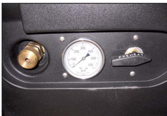
Spray pressure may be set here as well as pre-heating of the cleaning solution.
